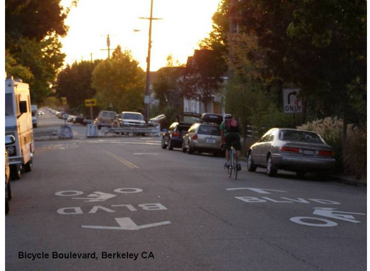
A Bicycle Boulevard in Berkeley CA: Motor vehicle through traffic is diverted to parallel streets.
