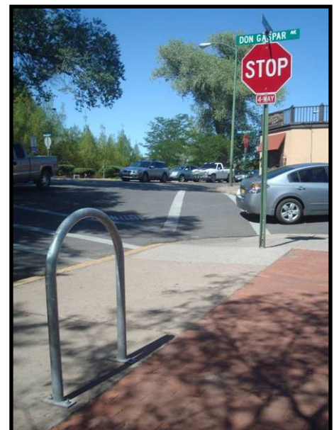
Key downtown locations that received loop racks under a special City initiative several years ago included the Plaza, City Hall, DeVargas Park, and the corner of Alameda and Don Gaspar (above). This inverted “U” design conforms with new guidance from APBP and AASHTO.
