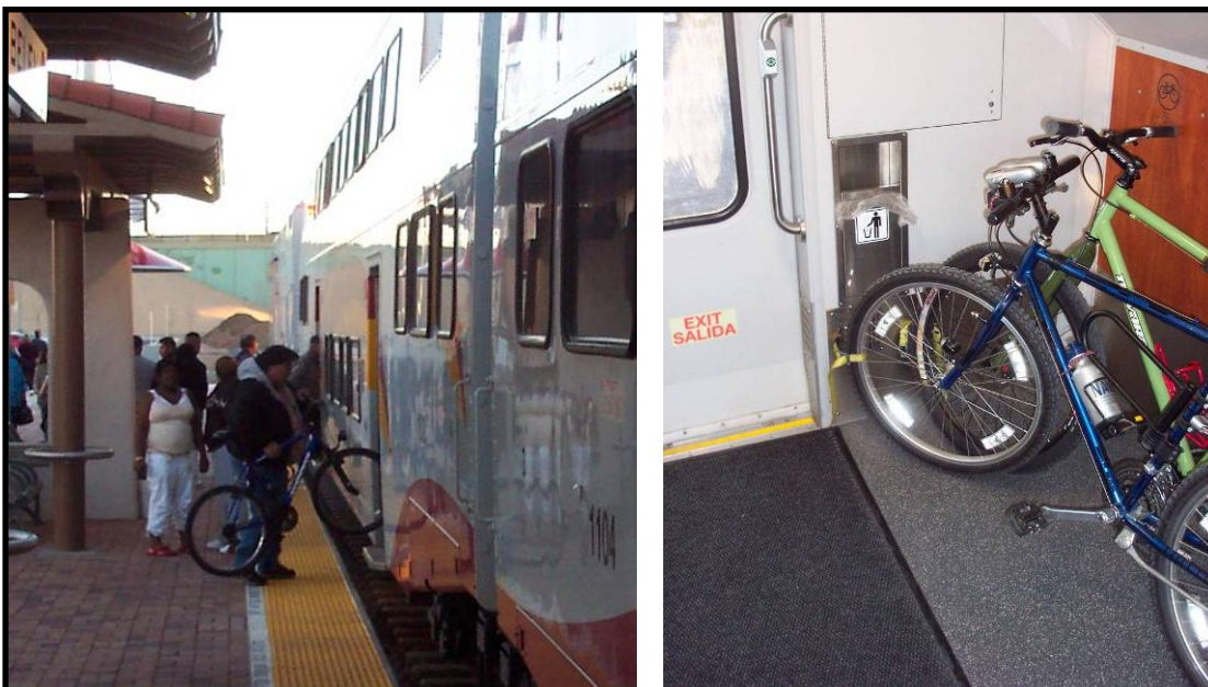
A Rail Runner passenger boards the train at a designated entrance (left). Space is reserved for a minimum of two bicycles per car (right); in practice several more bicycles may fit.
