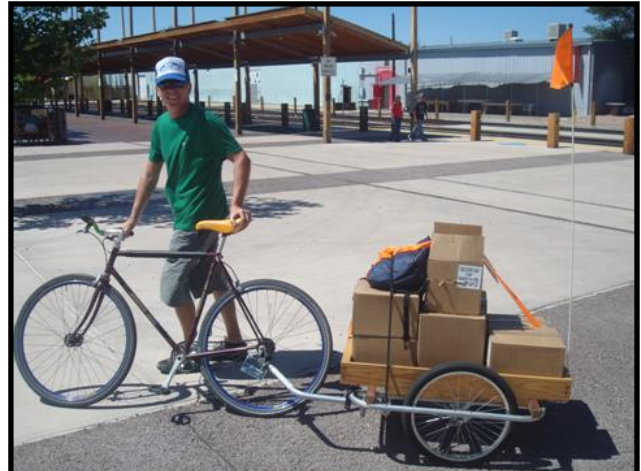
This bike and trailer combination can haul up to 250lbs. of deliveries at a time for Creative Couriers.
