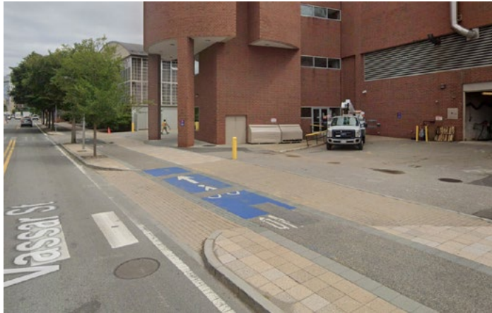
Protected bike facility in Cambridge utilizing high-contrast pain and a raised bike lane.
