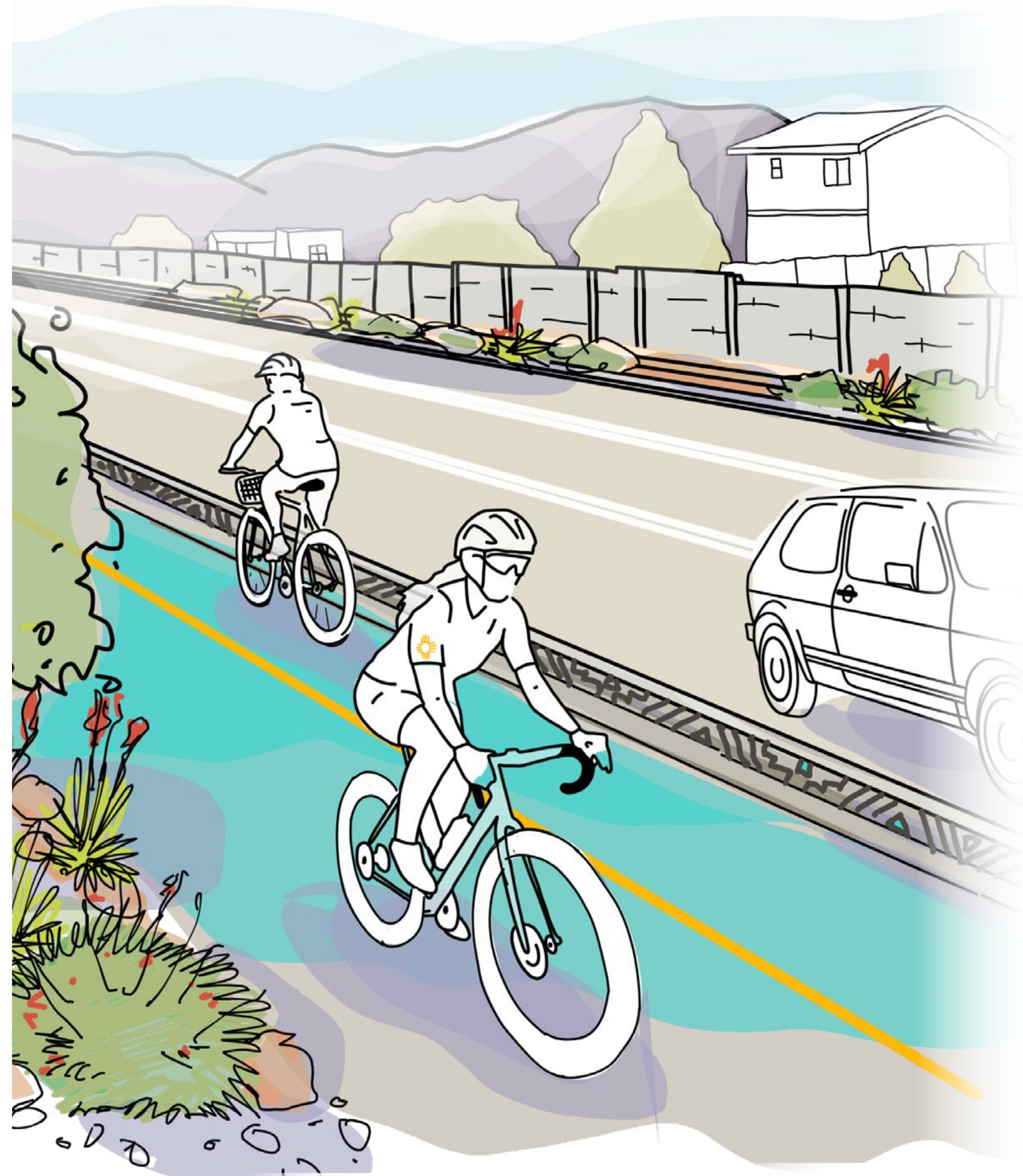
Painted curb stops featuring Native American patterns and vibrant turquoise pavement are relatively inexpensive options to incorporate a unique Santa Fe design element into safer bike facilities.
