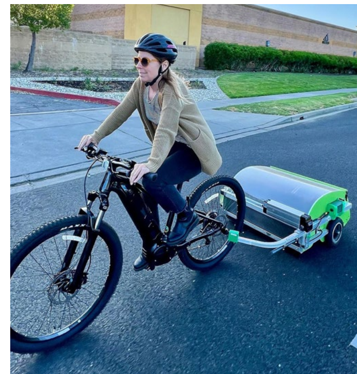
Pedal powered sweepers are a cheaper alternative, fulfill maintenance needs in cities with lower miles of bicycle facilities, and are a good opportunity to contract out with a community bike group.
