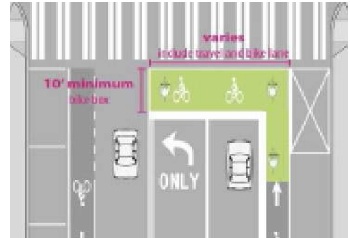
Figure 4.10: The 'bicycle box' allows a bicyclist to take a position in front of motor vehicles at an intersection which improves motorist awareness. Source: Toole Design Group
