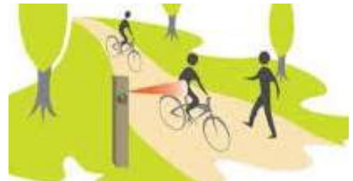
Figure 4.9: The Eco Counter 'Pyro' utilizes infrared sensors to record bicycle and pedestrian traffic. Source: Eco Counter
