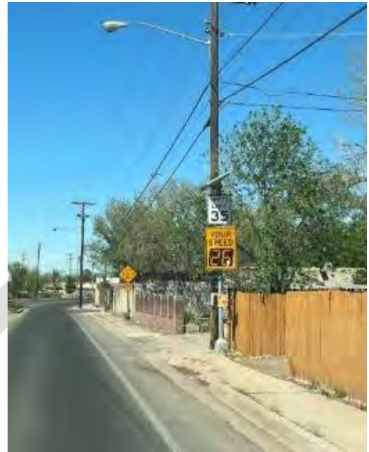
Figure 13. Radar speed feedback signs encourage speed limit compliance (Source: FHWA, 2022)
