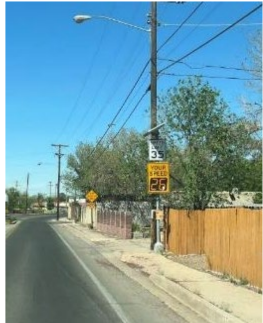
Figure 13. Photograph. Radar speed feedback signs encourage speed limit compliance (Source: FHWA, 2022).
