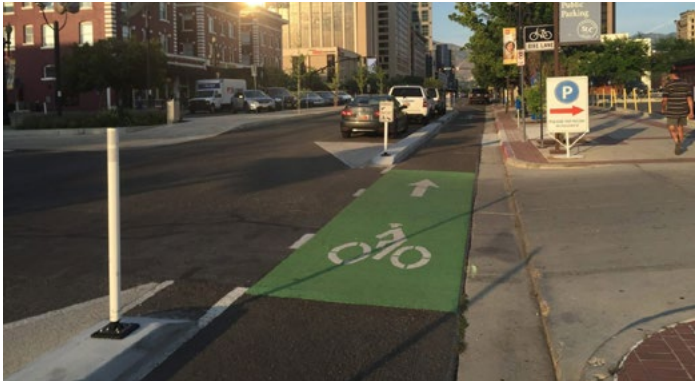
An example of green pavement used to highlight a bicycle facility at a driveway.
