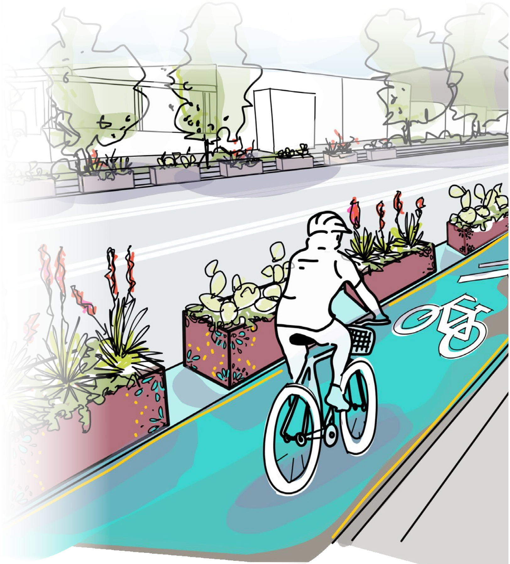
Planters featuring perforated steel design elements can serve as protective barriers while incorporating distinctive Santa Fe design motifs.
