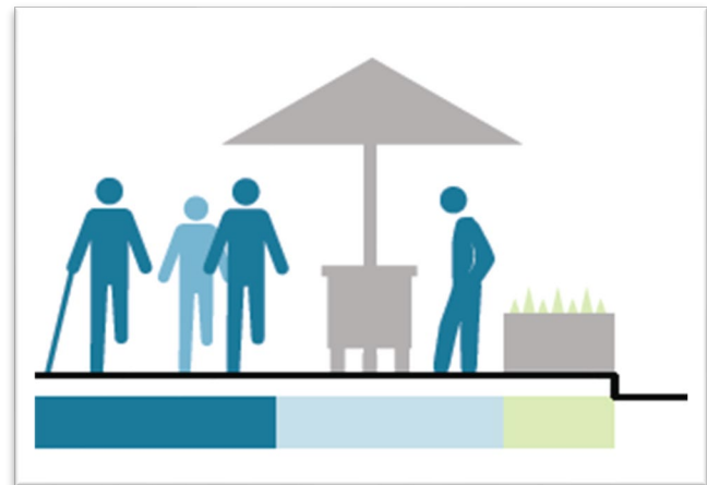
Figure 16: Planter Barrier in the Flexible Zone.
