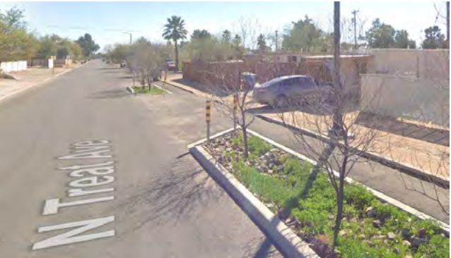
Bike facility improvements in Tuscon utilizing raised medians and other mea- sures to reduces conflicts at driveways and intersections.
