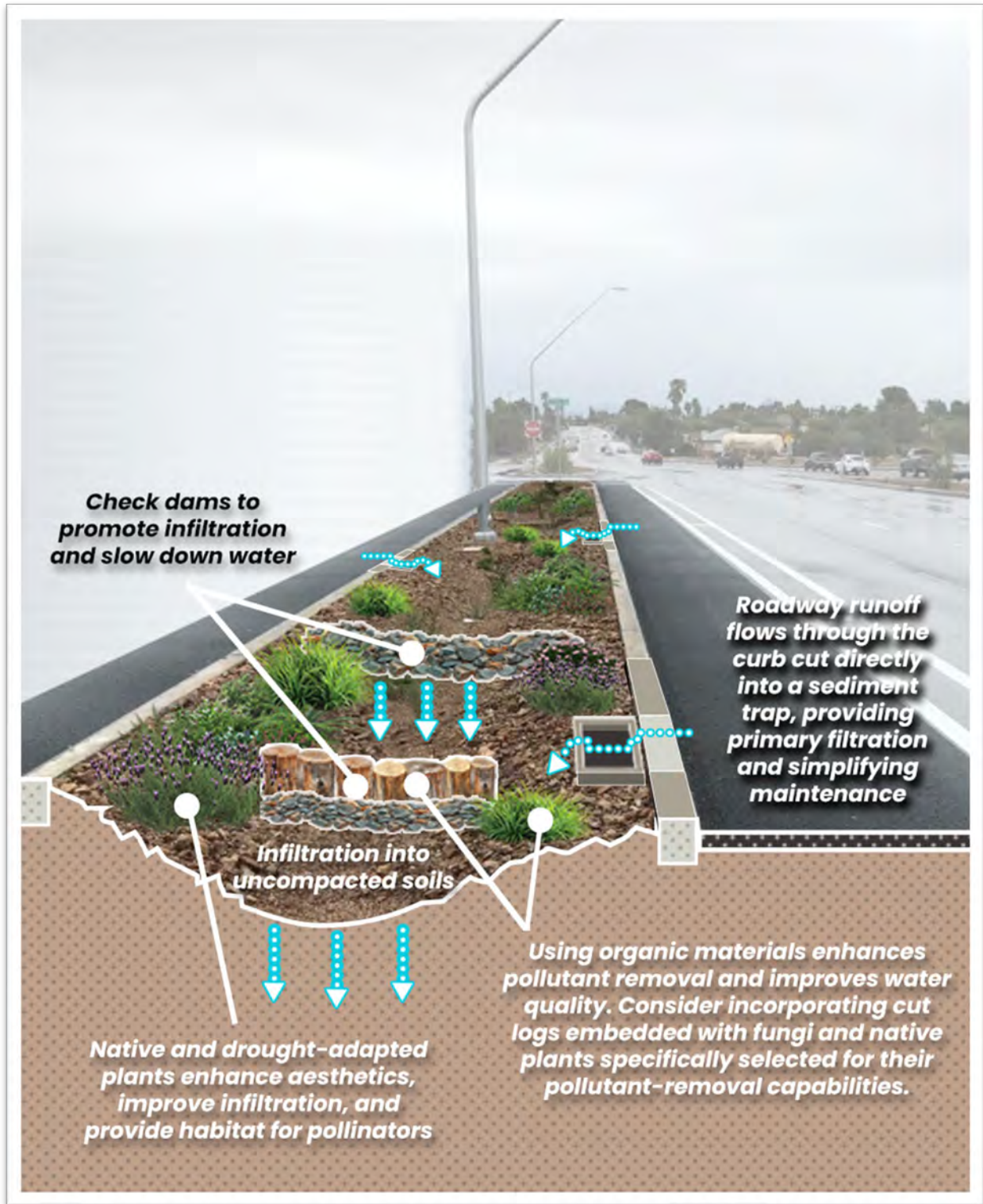
Figure 62: Bioretention Basin Diagram
