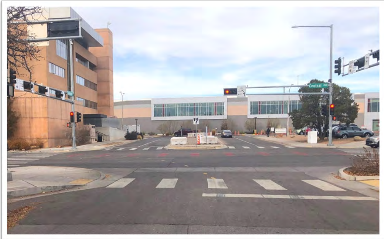
Figure 56: Curb Extension at Signalized Intersection
